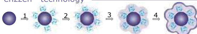
Figure 1: PER001 manufacturing steps. The enzyme is immobilized on non-porous silica nanoparticles (1), then organosilanes building blocks are self-assembled at the surface of the enzyme (2) and a polycondensation reaction produces a soft layer of controlled thickness (3). Finally, a biocompatible coating is added on the nanomedicine (4).
